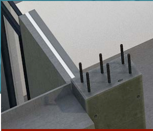
Thermally insulated triple outer walls
